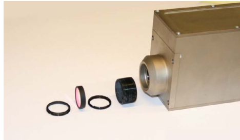
Fig. 4: Inserting a laser blocking filter in front of the detector
