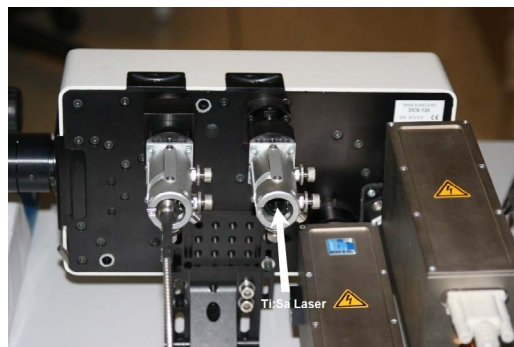
Fig. 2: Input of the Ti:Sa laser into the DCS-120 scanner
